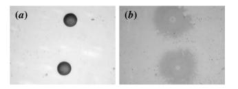
Figure 1. Optical micrographs (x100) of ink-jetted droplets on fluoro treated PET (Agfa). (a) surfactant containing jet ink (UGE 5529) with average drop diameter of 161  $\mu$ m, (b) model jet ink (U3285) without surfactant with average drop diameter of 424  $\mu$ m.
